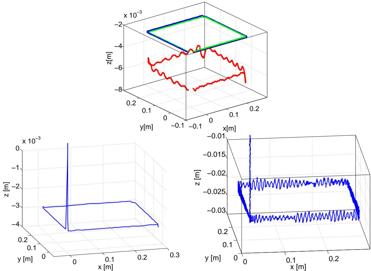
Figure 5: Measurement of the path that is cut into the soft model material (top) and simulation results for two different parameter sets (bottom). Note that the cut path is measured in terms of inboard, outboard and bottom line of the cut channel.
