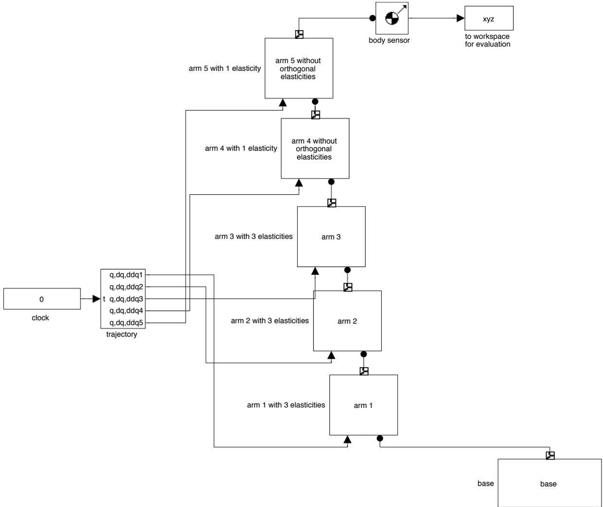
Figure 3: The model of the robot consists of blocks, each with one joint with one or three elasticities and dampers and one stiff link (“arms”).
