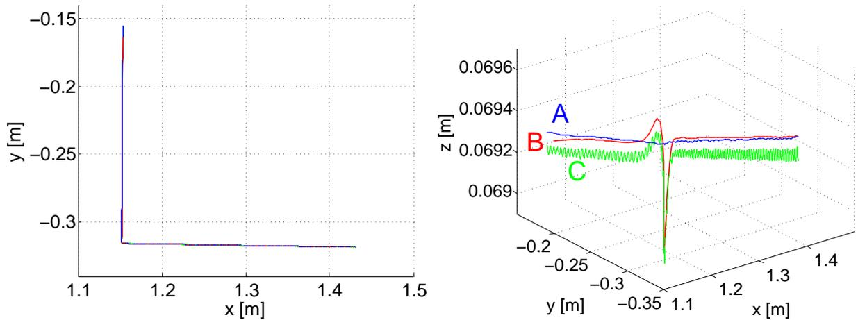
Figure 4: Path of the tool center point at a corner of its trajectory: From a computational model without any elasticity (A; blue), with joint angle elasticity (B; red), and with both joint angle and tilting elasticities (C; green). Note the different scales of the axes.
