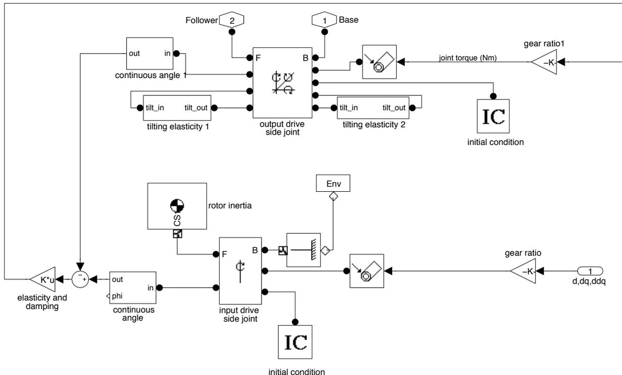
Figure 2: The first three joints are modeled to have elasticities and damping orthogonal to the direction of motion (“tilting elasticity 1” and “tilting elasticity 2”) besides the elasticities and damping in direction of motion.
