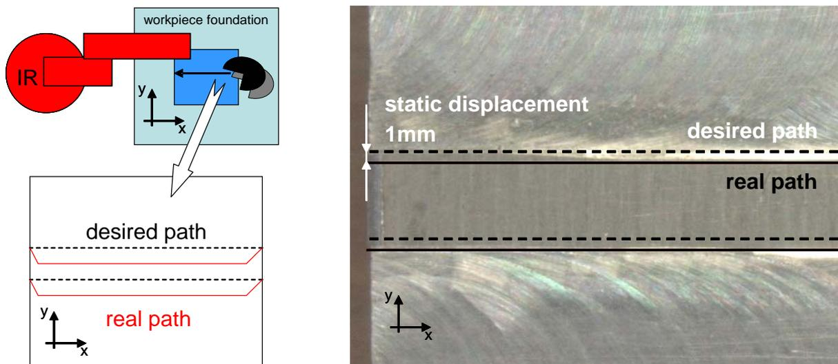
Figure 1: The path of the tool center point shows an offset from the desired path. This is mainly due to the elasticity of the joints.
