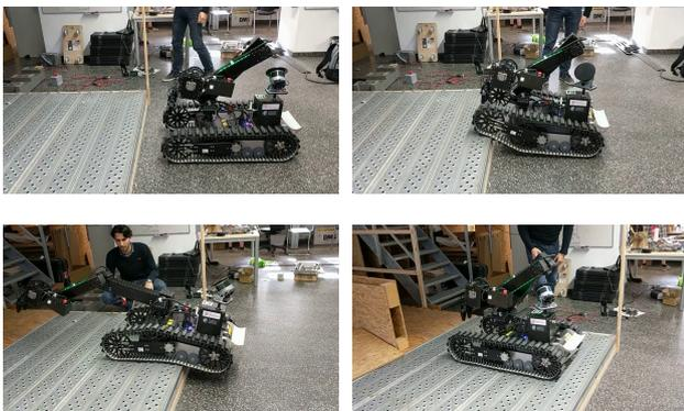
Figure 9 Visualization of the whole-body motion plan on the real *Hector Tracker* robot
