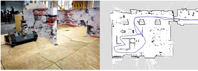
(a) ExR-1 robot in the rescue (b) Generated map segment of the robot test arena with the robot trajectory in blue.
