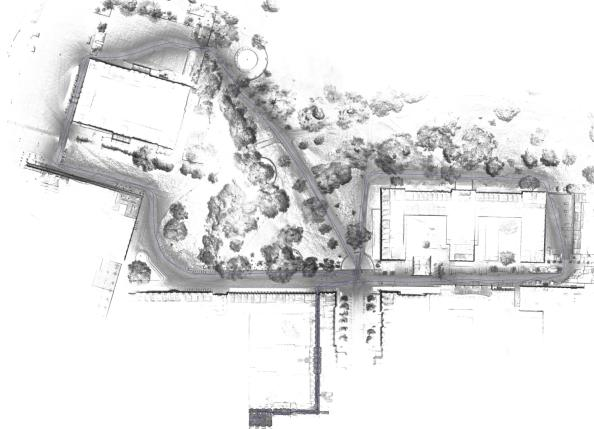
(c) Projection of the generated point cloud. The color encodes the point density.
