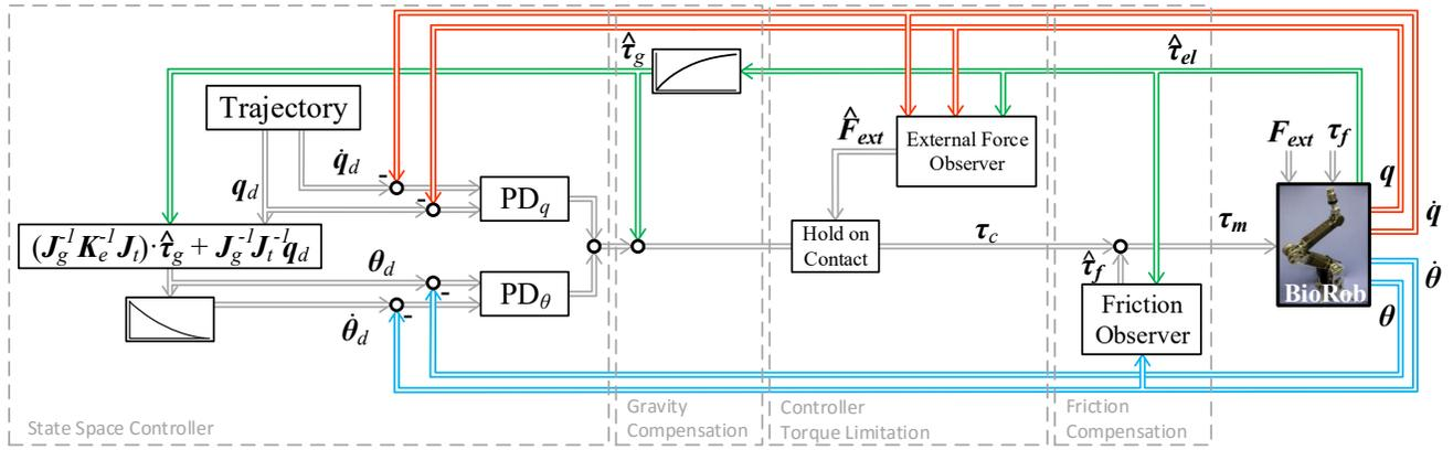
Fig. 4. State space controller extended with friction compensation  $\hat{\tau}_f$ , torque limitation based on external force estimation  $\hat{F}_{ext}$  and feedback of estimated joint torque  $\hat{\tau}_{el}$  for gravity compensation and equilibrium controlled stiffness.
