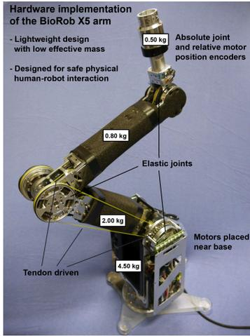
Fig. 1. Hardware implementation of a BioRob X5 arm with four elastically actuated joints (fifth joint not used). The robot arm has a reach of about 75cm, weighs 7.8kg including power electronics and has a nominal payload of 500g. The schematic actuation principle with springs embedded in the joint pulley is depicted in Fig. 2.
