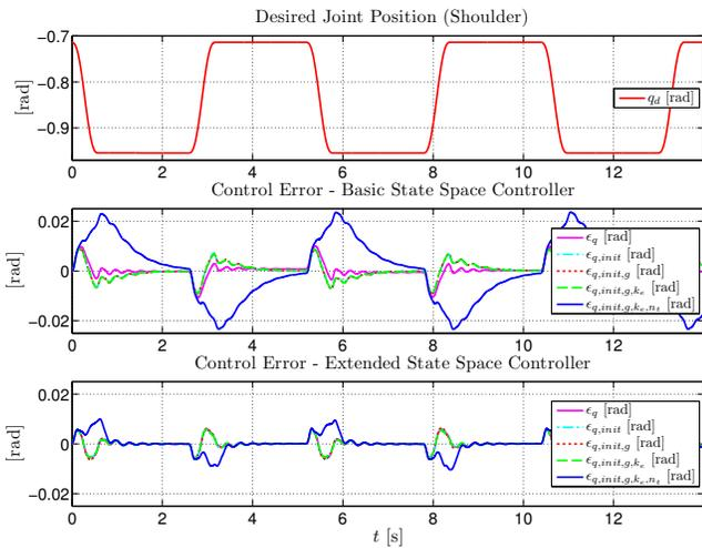
Fig. 5. Desired shoulder trajectory  $q$  and the resulting control position error containing the various model inaccuracies for the basic state feedback controller with gravity compensation as well as for the extended state feedback controller with friction compensation, equilibrium controlled stiffness and feedback of the estimated elastic torque, executed in simulation.
