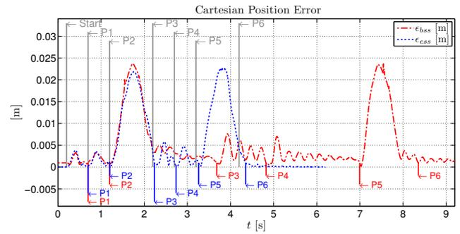
Fig. 8. Comparison of the Cartesian position error and execution time of the basic  $\epsilon_{bss}$  and extended state space controller  $\epsilon_{ess}$ , during Inch-Foot trajectory execution on the real robot. Marks P1-P6 indicate the trajectory point's planned (gray) and executed reaching time.
