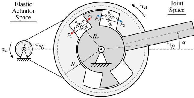
Fig. 2. Model of the elastic transmission adapted from [21]. Springs are placed in pulley. Parameters are: elastic actuator torque  $\tau_{el}$ , elastic actuator joint torque  ${}^j\tau_{el}$ , spring forces  $F_i$ , spring stiffness  $k_i$ , spring damping  $d_i$ , motor pulley radius  $r$ , joint pulley radius  $R$ , spring radius  $R_s$ , angular joint position  $q$ , angular motor position  ${}^e\theta$  with respect to the elastic actuator and joint  ${}^j\theta$ .
