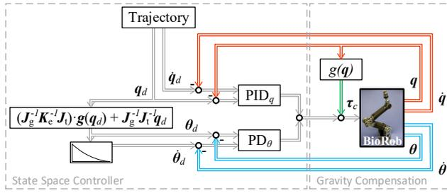
Fig. 3. State space controller with feedback of whole robot state  $(q, \dot{q}, \theta, \dot{\theta})^T$ , desired motor position  $\theta_d$  and velocity  $\dot{\theta}$  computation, as well as model based gravity compensation producing the control torque  $\tau_c$ .
