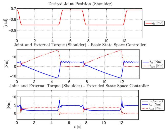
Fig. 6. Comparison of the estimated external joint torques  $\hat{\tau}_{ext}$  and elastic joint torques  $\hat{\tau}_{el}$  of the basic and extended state space controller, executed in simulation. A "inContact" value of 10 indicates that the controller is in contact mode.
