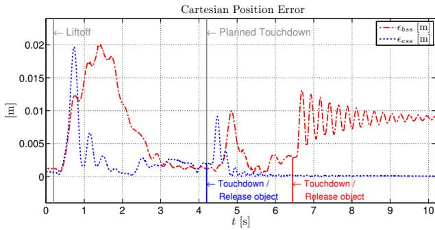
Fig. 7. Comparison of the Cartesian position error and execution time of the basic  $\epsilon_{bss}$  and extended state space controller  $\epsilon_{ess}$ , during lifting a 500g object, executed on the real robot.
