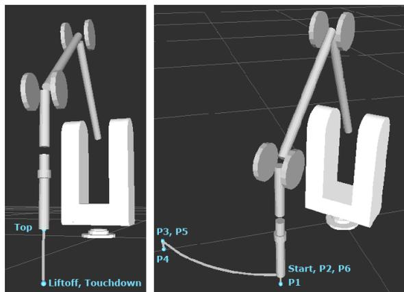
Fig. 9. Visualization of the planned pick and Inch-Foot-Inch trajectory, used for experiments.
