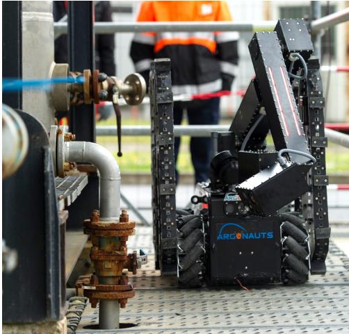
Fig. 1 Current ARGONAUTS robot autonomously inspecting a valve in an industrial plant during the 2nd ARGOS Competition. The sensor arm is used to obtain a close-up view of the object of interest.
