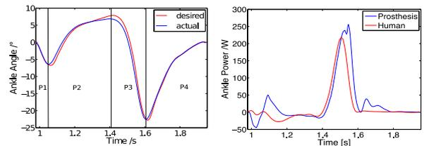
Figure 3: (a) Ankle angle; (b) Ankle power
