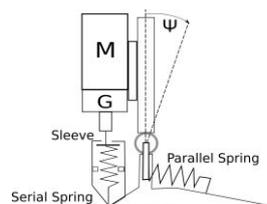
Figure 1: Mechanical setup of the ankle-foot
