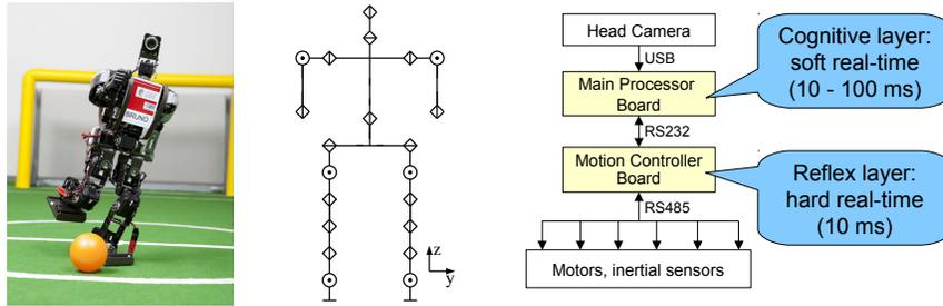
Fig. 1: Autonomous humanoid robot *Bruno* (©K. Binner) kicking a ball (left), kinematic robot structure (middle), main layers of information processing (right).
