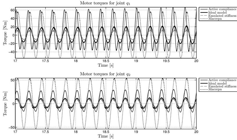
**Fig. 10.** Motor torques required for the desired trajectories  $q_1$  and  $q_2$  generated by the ideal system with online adaptable spring stiffness, active compliant system, Macepa actuators and emulated spring stiffness technique.
