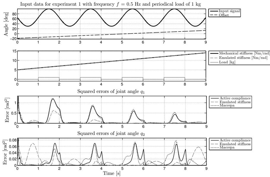
**Fig. 6.** Experiment 1, i.e. sine wave as reference input for both joints with given emulated and mechanical spring stiffness with a step frequency of 0.5 Hz, is repeated additionally with ground contact which is achieved by a periodical load of 1 kg.
