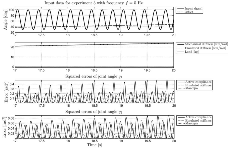
**Fig. 7.** Experiment 3: Similar setup as in Experiment 1, sine wave as reference input for both joints with given emulated and mechanical spring stiffness with an increased frequency of 5 Hz without ground contact.
