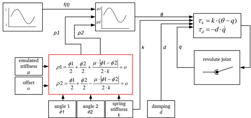
**Fig. 3.** Schematic of the feedforward controlled emulated spring stiffness technique.
