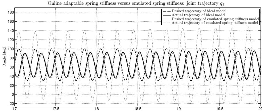
**Fig. 9.** Desired and actual trajectories obtained by the ideal system with online adaptable spring stiffness for joint  $q_1$  versus the input and response trajectories obtained by the emulated spring stiffness technique.
