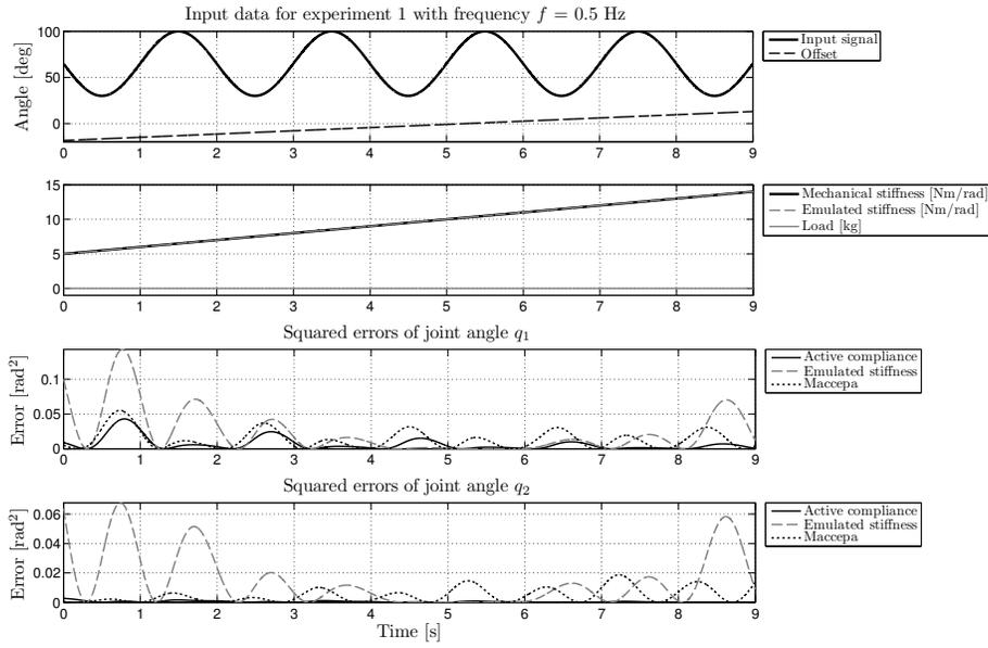
**Fig. 5.** Experiment 1: Sine wave as reference input for both joints with given emulated and mechanical spring stiffness with a step frequency of 0.5 Hz. The experiment is performed without ground contact.
