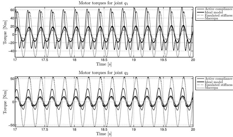
**Fig. 10.** Motor torques required for the desired trajectories  $q_1$  and  $q_2$  generated by the ideal system with online adaptable spring stiffness, active compliant system, Macepa actuators and emulated spring stiffness technique.
