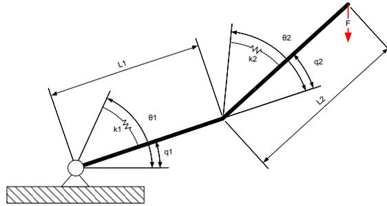
**Fig. 4.** Both joints of the 2-DOF arm are actuated by rotary SEAs. The variables  $\theta_1$  and  $\theta_2$  represent the motor positions while  $q_1$  and  $q_2$  stand for the joint positions.  $k_1$  and  $k_2$  denote the predefined mechanical spring stiffness of the SEAs.
