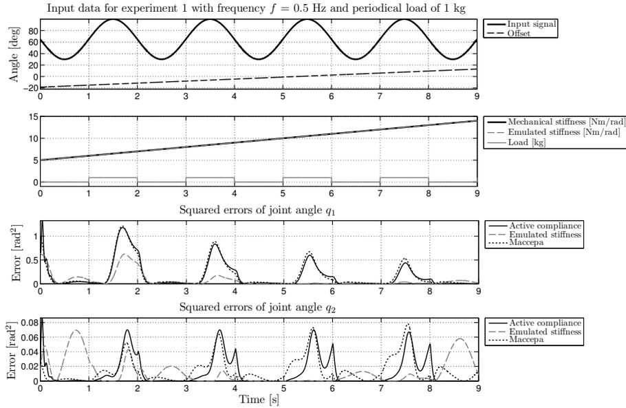
**Fig. 6.** Experiment 1, i.e. sine wave as reference input for both joints with given emulated and mechanical spring stiffness with a step frequency of 0.5 Hz, is repeated additionally with ground contact which is achieved by a periodical load of 1 kg.
