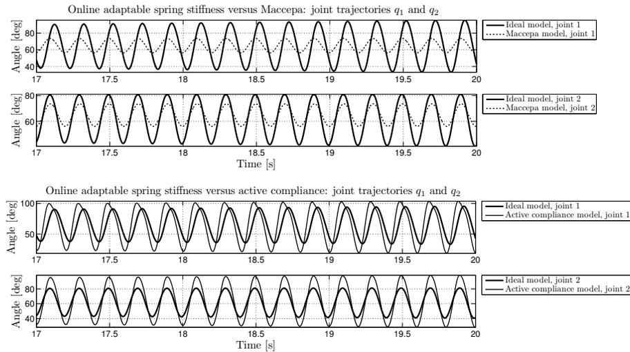
**Fig. 8.** Actual trajectories respectively measured responses obtained by the 2-DOF arm with on-line adaptable spring stiffness are compared to the responses obtained by Maccopa actuation for joints 1 and 2 in the uppermost plot. In the lower plot the responses of the ideal system with online adaptable spring stiffness are compared to the responses of the active compliant system.
