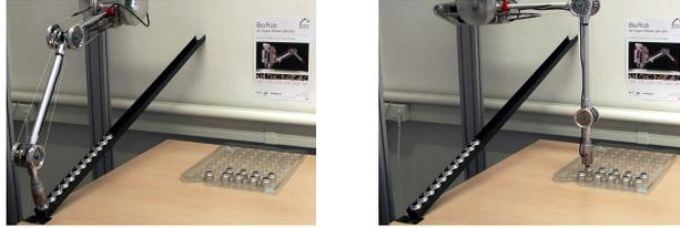
Fig. 10. Pick and place application with the BioRob robot arm [2].
