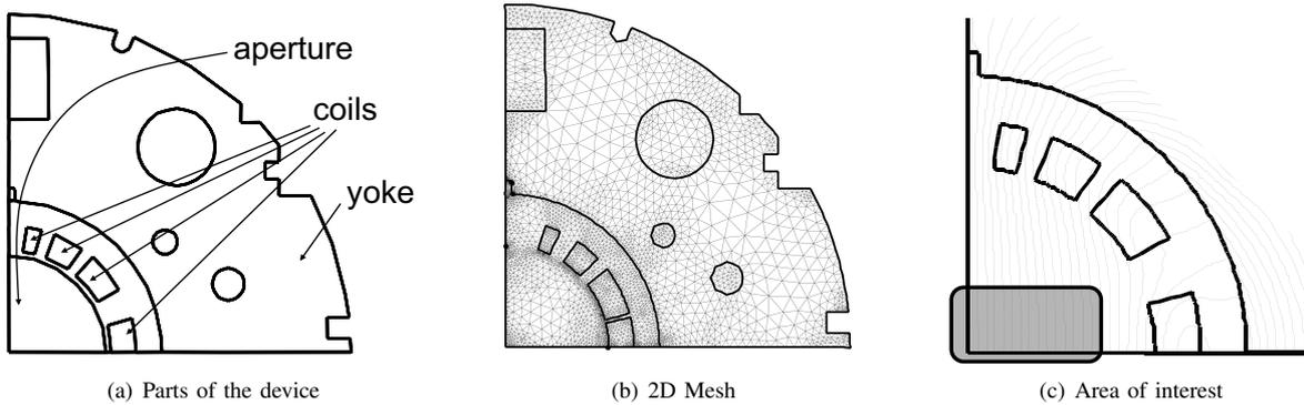
Fig. 1. 2D design optimization problem of the location and size of the coil blocks (a), the resulting mesh of a considered design (b), and the visualization of the computed electromagnetic field in the aperture of the magnet (c).
