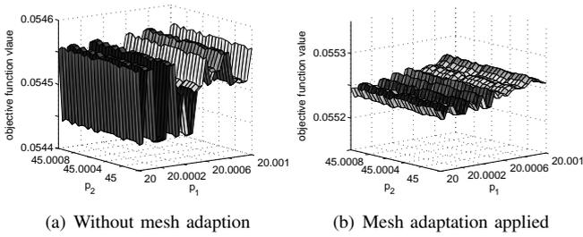
Fig. 2. Comparison of the optimization surface smoothness without (a.) and with (b.) one mesh adaption step.
