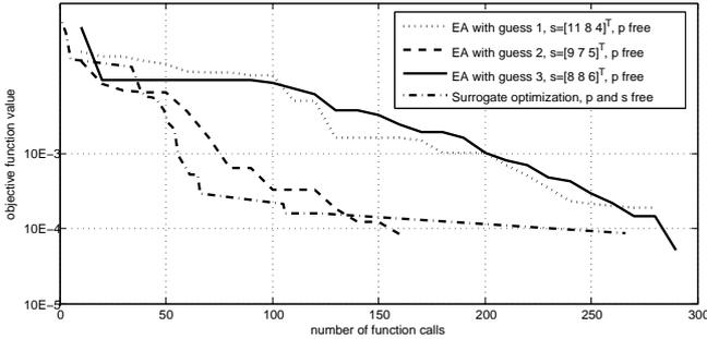
Fig. 3. Progress of three different optimization methods, three runs with an Evolutionary Algorithm, each with a different discrete design and only free continuous design variables, and one run with the proposed surrogate optimization method, with free discrete and free continuous design variables.
