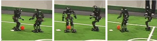
Fig. 5. Cooperative team behavior during the 2 on 2 humanoid robot soccer game for 3rd place at RoboCup 2006: Both robots detect the ball, the left robot is closer to the ball, gets the role "striker" and continues to approach the ball while the right robot obtains the role "supporter" and steps back.
