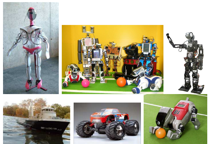
Fig. 5. Selected robot systems running applications based on RoboFrame in the authors research group. Upper row: humanoid robot Lara (left) actuated by artificial shape memory alloy muscles, several humanoid, legged and wheeled robots (middle), autonomous humanoid robot Bruno (right). Lower row (from left): robotic boot, robotic offroad vehicle, new four-legged robot.
