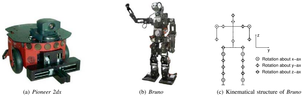
Fig. 1. Strongly heterogeneous robots in this application: Wheeled robot Pioneer 2dx and humanoid robot Bruno .
