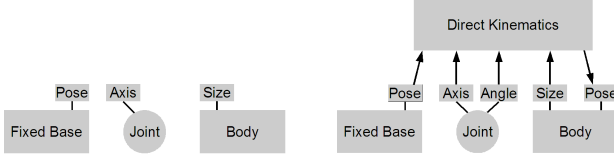
Fig. 3. Left: Modeling of a 1 DOF robot arm. Only the known properties are added to the model. Right: When connecting a simulation algorithm (here: direct kinematics) to the model, additional properties needed or calculated by the algorithm are added to the model.
