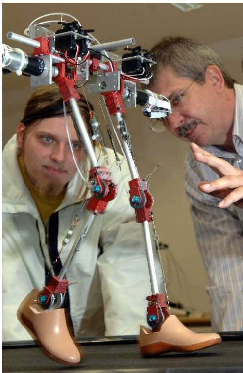
Fig. 1. The JenaWalker II bipedal robot testbed.
