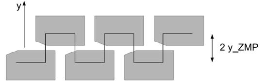
Fig. 3. The desired ZMP position  $y_{ZMP}$  (solid line) during a walking motion.  $y_{ZMP}$  is always in the middle of the standing foot.
