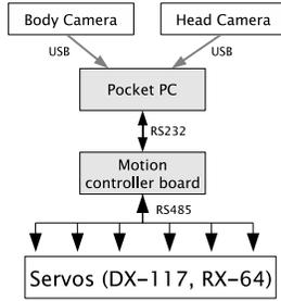
Fig. 2. Flow chart of information data stream in the semi-distributed system.
