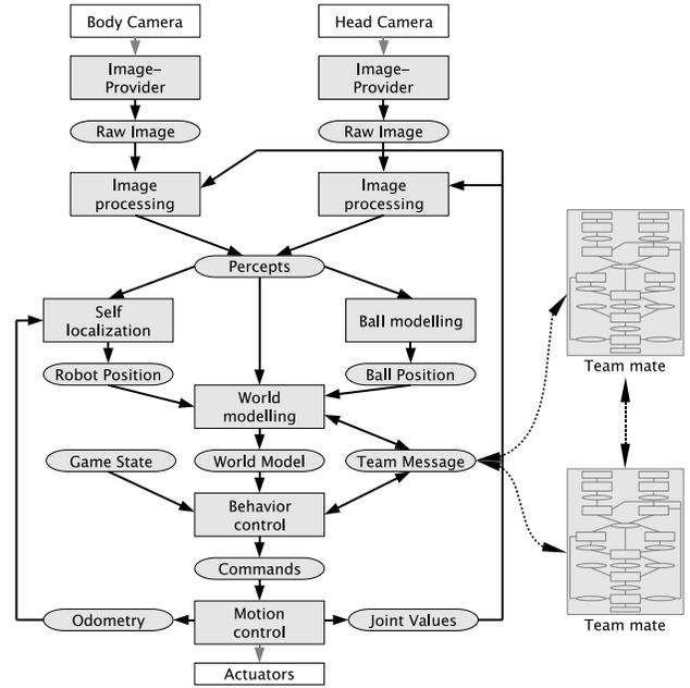
Fig. 7. Overview of modules (rectangles) and exchanged messages (ellipses) of the control software. White blocks are sensors or actuators, gray blocks are modules executed on the Pocket PC.
