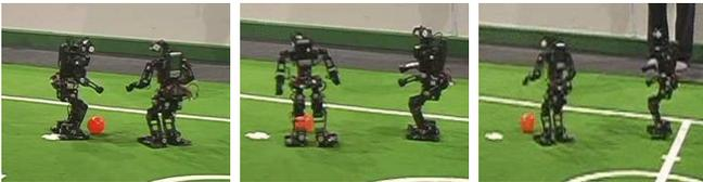
Fig. 10. Cooperative team behavior during the 2 on 2 humanoid robot soccer game for 3rd place at RoboCup 2006: Both robots detect the ball, the left robot is closer to the ball, gets the role "striker" and continues to approach the ball while the right robot obtains the role "supporter" and steps back.
