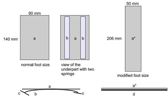
Fig. 6. Two different foot design for walking on a rough terrain. In the left design, two springs (b) are attached on the foot plate (a). On each spring, two moveable plates (c) are mounted to avoid stumbling. In the right design, the foot (a\*) is enlarged in the length and shortened in the width. On the underpart, a soft material (d) is added.
