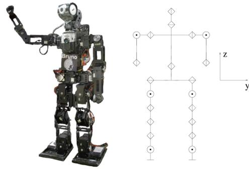
Fig. 1. The 55cm tall, autonomous humanoid robot Bruno (left) which is based on the Hajime Robot HR18 and its kinematic structure (right).
