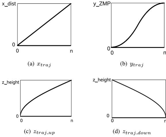
Fig. 4. Trajectories for walking motion for  $x$ ,  $y$  and  $z$ .
