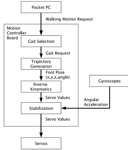
Fig. 5. Structure and dataflow of motion generation. Motion requests made by the robot's behavior control are processed in a series of steps on the motion controller board. After selecting an appropriate gait for the requested motion, the trajectory for the feet is generated using ZMP theory. Using inverse kinematics, the necessary angles for the joints are calculate. To improve walking stability, inertial sensors are used to modify these angles.
