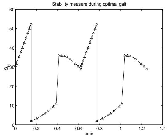
Fig. 2. Stability index  $S_H$  for optimized gait of a quadruped moving forward at 0.67 m/s and duty factor  $\beta = 0.5$  based on a full three-dimensional dynamical model.
