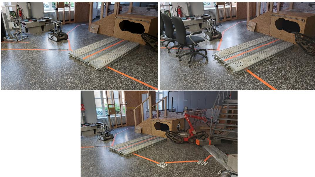
Figure 6.1.: (Top Left) The robot has the options to drive across or around the obstacle. (Top Right) The path around the obstacle is blocked, and the robot has to cross the obstacle. (Bottom) The robot should avoid the first obstacle but cross the second.
