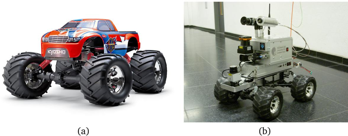
**Figure 5.1:** Vehicle: (a): Unmodified Kyosho TwinForce R/C car (Image from [38]) (b): The experimental platform created by modification of a TwinForce R/C car.
