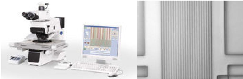
**Image 3 - Wafer Inspection System MX61A and a deep ultraviolet image of a CPU**
