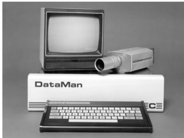
Image 1 - DataMan - first OCR<sup>1</sup> system developed by Cognex Corporation in 1982
