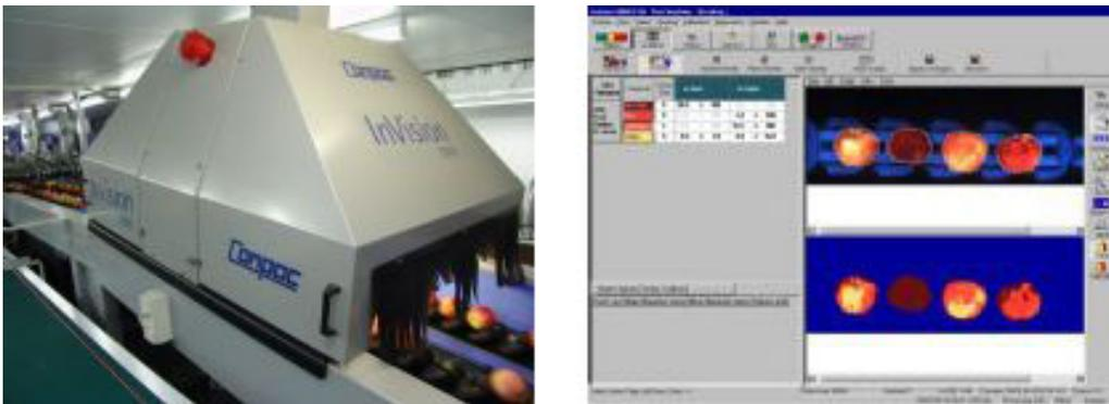
Image 2 - Sorting System InVision 5000 and graded apples in software
