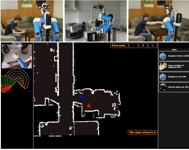
Fig. 2. Illustration of our task-level teleoperation interface. Top left: A user composes a task. Bottom/top middle: The robot grasps an object. Top right: The robot delivers the object.
