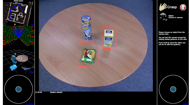
Fig. 1. Skill and body-level GUI with a view selection column on the left, a main view in the center, a configuration column on the right, and a log message window on the bottom center. Motion is controlled directly with two joystick control UIs.
