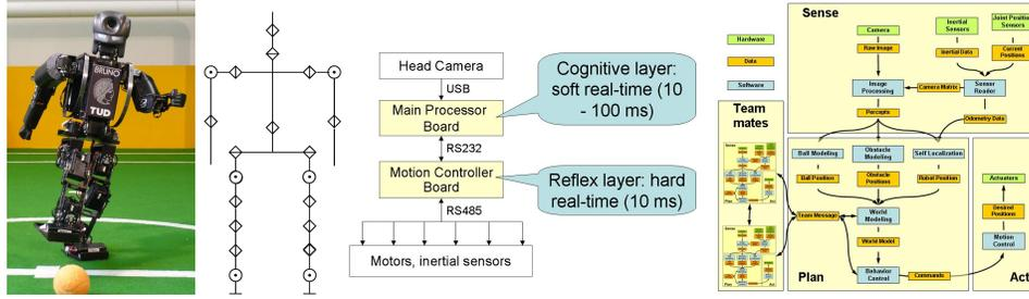
**Fig. 1.** Autonomous humanoid robot *Bruno* (with designed head) kicking a ball (left), kinematical robot structure (middle left), main layers of information processing (middle right) and control architecture (right).
