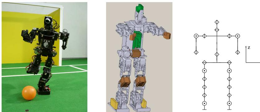
Autonomous humanoid robots *Bruno* and *Jan* kicking a ball (model 1, left), CAD-drawing of new robot (model 2, middle) and kinematical structure of both robots (right).
