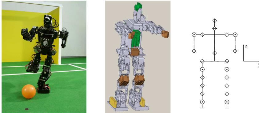
**Fig. 1.** Autonomous humanoid robot *Jan* (model 1) kicking a ball (left), CAD-drawing of new robot (model 2) (middle) and kinematical structure of both robots (right).
